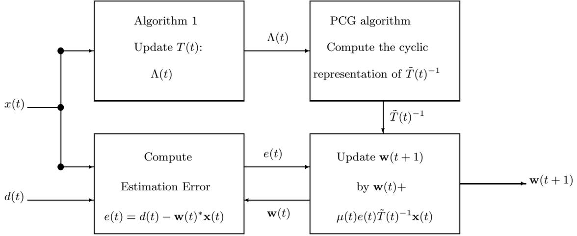
FIG. 1. Block Diagram of the FFT-based LMSN Algorithm.
