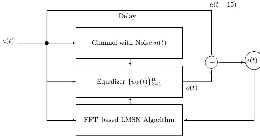
FIG. 8. The Equalization Problem used for Simulation.
