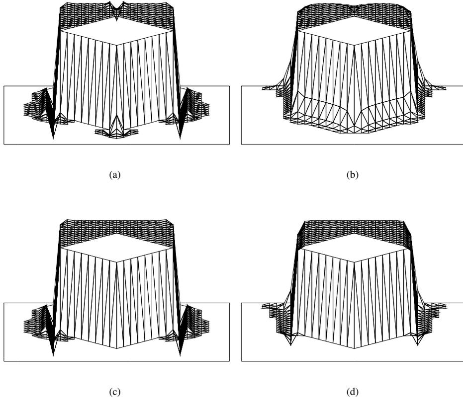
FIG. 7.3. Example 7.2, triangulation from Figure 7.1(a): (a) SUPG method with  $\tau$  from (2.2), (b) SOLD method with  $\tau$  from (2.2) and SOLD term (3.1), (3.2), (c) SUPG method with  $\tau$  defined by (4.1), (d) SOLD method with  $\tau$  defined by (4.1) and SOLD term (3.1), (3.2).
