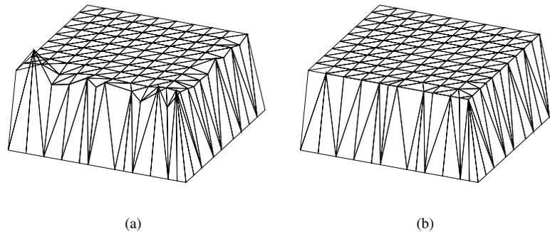
FIG. 5.2. *Example 5.1, SUPG solutions computed on the triangulation from Figure 5.1(c): (a)  $\tau$  defined according to Madden and Stynes [14], (b)  $\tau$  defined by (4.1).*
