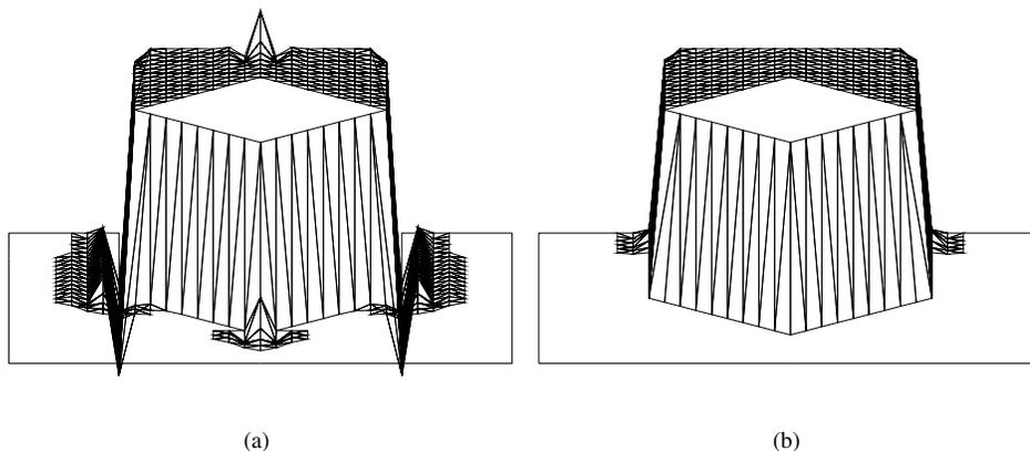
FIG. 7.4. Example 7.2, triangulation from Figure 7.1(b), SUPG method: (a)  $\tau$  defined by (2.2), (b)  $\tau$  defined by (4.1).
