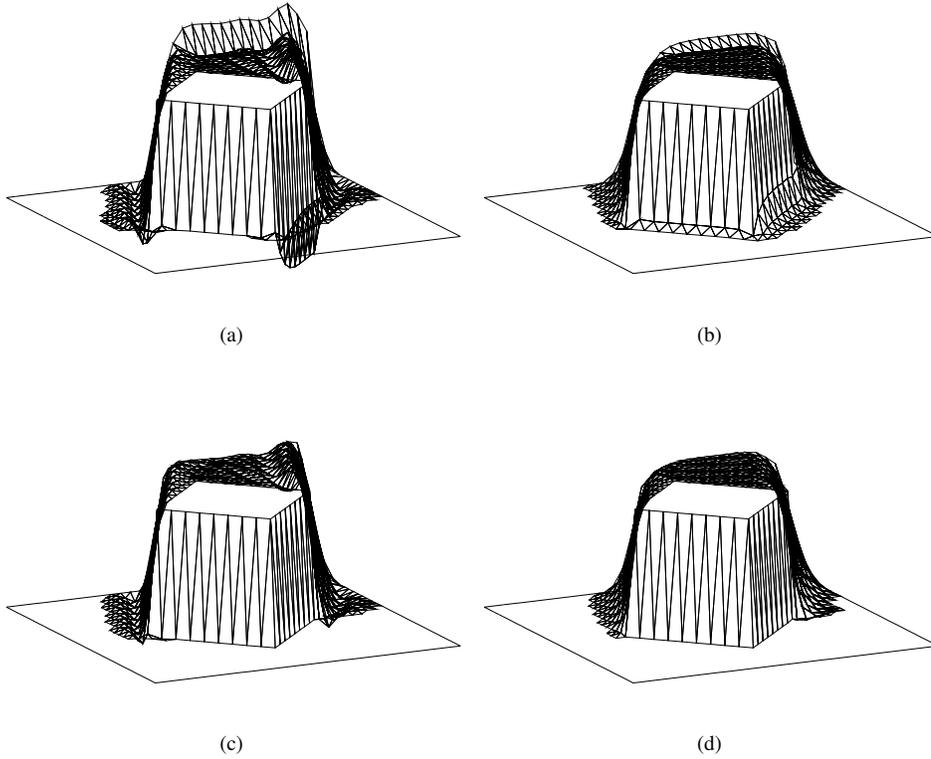
FIG. 7.2. Example 7.1, triangulation from Figure 7.1(a): (a) SUPG method with  $\tau$  from (2.2), (b) SOLD method with  $\tau$  from (2.2) and SOLD term (3.1), (3.2), (c) SUPG method with  $\tau$  defined by (4.1), (d) SOLD method with  $\tau$  defined by (4.1) and SOLD term (3.1), (3.2).
