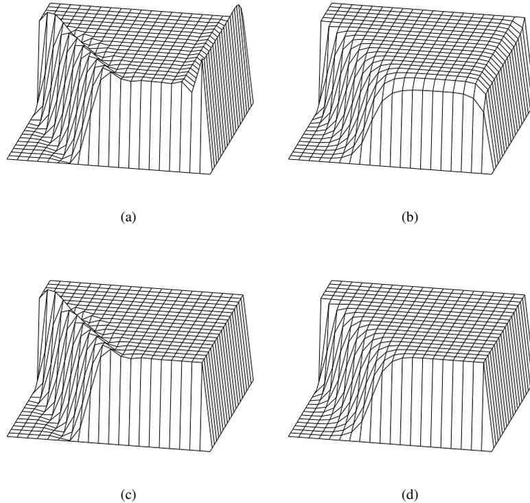
FIG. 6.1. Example 6.1,  $21 \times 21$  triangulation of the type from Figure 5.1(b): (a) SUPG method with  $\tau$  from (2.2), (b) SOLD method with  $\tau$  from (2.2) and SOLD term (3.1), (3.2), (c) SUPG method with  $\tau$  defined by (4.1), (d) SOLD method with  $\tau$  defined by (4.1) and SOLD term (3.1), (3.2) applied away from the boundary layers.
