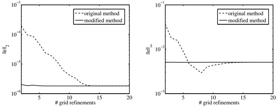
FIG. 4.2. *Behavior of the error of the original method and of our modification. Using the original method both, the error in the 2-norm and in the  $\infty$ -norm, depend heavily on the number of grid refinements. The accuracy converges to the accuracy of our modification, that is almost independent of the number of refinements.*
