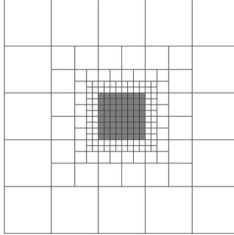
FIG. 2.1. Coarsened grid in 2D. Highlighted is the original fine grid, in which the solution is of interest.
