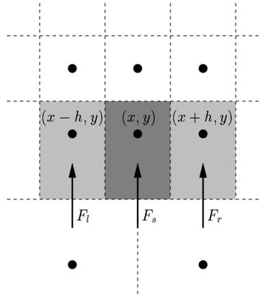
FIG. 2.2. Conservative discretization at the interface in 2D.
