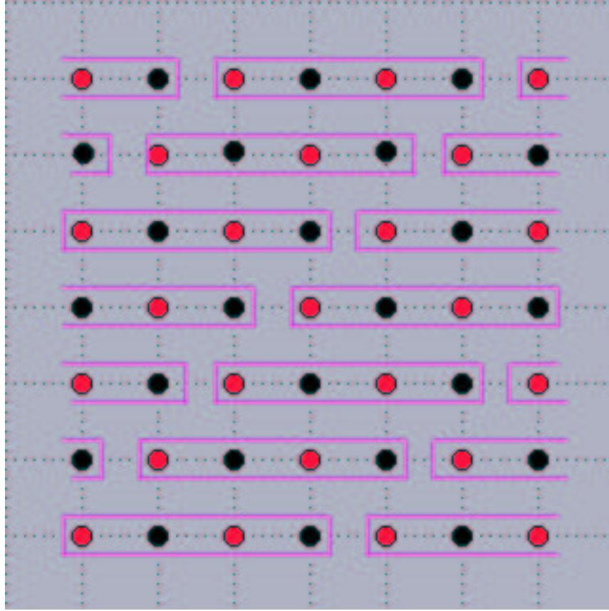
FIG. 4.2. Standard layout of the red-black Gauss-Seidel unknowns in memory for a cache-line size of 4.
