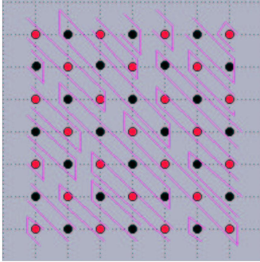
FIG. 4.4. The new layout of data in memory for Gauss-Seidel using the cache aware data layout scheme. Here too, the size of a cache-line is 4.
