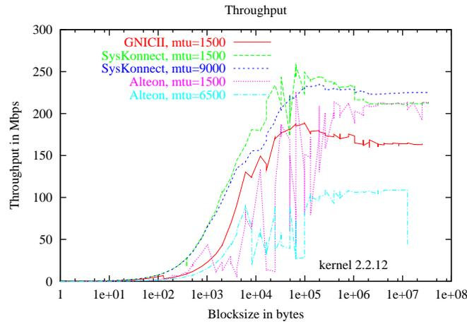
FIG. 6.2. *GNIC-II, Alteon & SysKconnect: MPICH Throughput*
