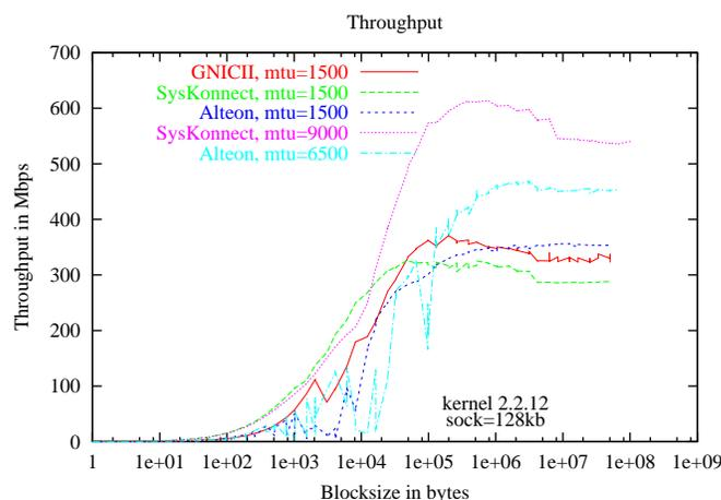
FIG. 4.5. *GNIC-II, Alteon, & SysKonnnect: TCP Throughput and Latency*
