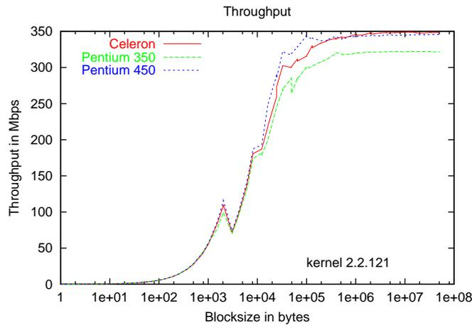
FIG. 4.2. Processors Comparison: Throughput
