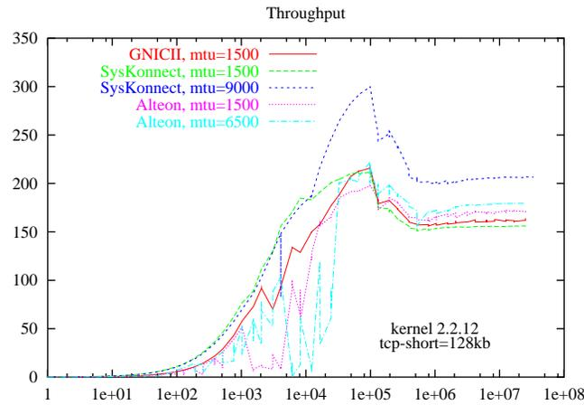
FIG. 6.1. *GNIC-II, Alteon, & SysKconnect: LAM Throughput*
