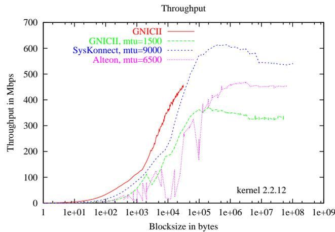
FIG. 5.1. GNIC-II: M-VIA Throughput
