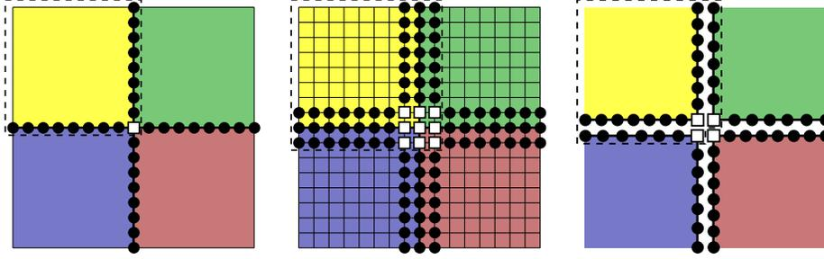
FIG. 2.2. Illustration of dofs and globs for left: conforming standard  $P^1$  finite element discretization, middle:  $C^2$ -continuous B-spline discretization (grid lines displayed), right: standard  $P^1$  discontinuous Galerkin discretization. White rectangles belong to the subdomain vertex, solid dots belong to subdomain edges; a dashed line marks the dofs of a subdomain.
