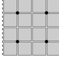
FIG. 3.1. Example where (3.1) is not sufficient to guarantee that  $\tilde{S}$  is definite; 2D Laplace problem with Dirichlet boundary conditions on the dashed line. A bullet indicates primal constraint on a subdomain vertex.
