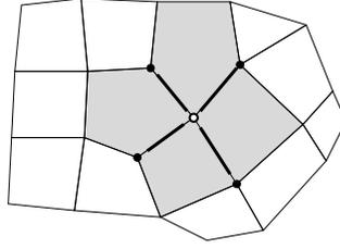
FIG. 3.2. Sketch of a vertex  $G$  (marked with  $\circ$ ) and the neighboring globs where constraints enforced in the associated space  $\tilde{W}_{\mathcal{N}_G}$  (marked with thick lines and black dots).
